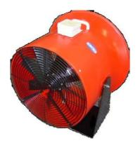
The Portable Axial Fan is specifically designed to provide air movement and ventilation in a variety of situations. The fan casing is moulded from plastic. The motor and bracket are aluminium and the adjustable pitch impeller is polypropylene. The high efficiency impeller with eight wings provides for a very high air flow of 6300 m<sup>3</sup>/hr.
